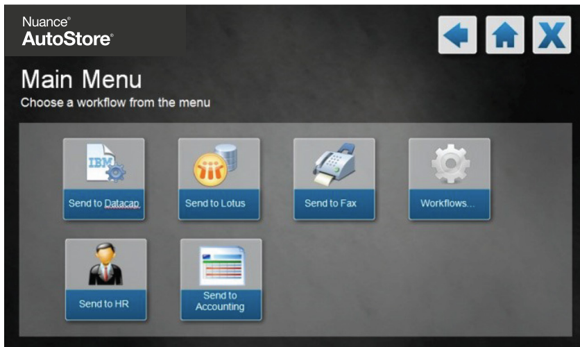
Figure 2: Workflow selection home screen. Personalized Mask on the front panel of a multifunction device
